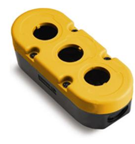
The ASI EP3C3AA000 is a rugged Control Station 3 Hole Enclosure designed to hold up to three 22mm pushbuttons, switches, or pilot devices. Constructed from durable yellow polycarbonate, it offers superior protection with IP65/IP69K and NEMA 4X ratings—perfect for harsh industrial environments. The enclosure's ergonomic, compact design simplifies installation while delivering reliable, maintenance-free operation for multifunction control setups.
