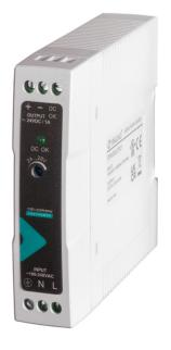
The XCSE1024W024VAA is a compact, single-phase DIN rail power supply designed for industrial automation and control panels. Delivering a stable 24 VDC output at 1 A, it supports a wide input range of 90–264 VAC or 127–370 VDC, making it ideal for global applications. Featuring high efficiency, full electronic protections, and DIN rail mounting, it's engineered for reliable performance in demanding environments.
