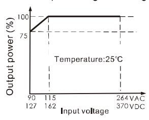
1.85-100VAC/120-140VDC input voltage derate input voltage on the base of temperature derating. 2. The use of product is in a natural cold environment. If in a closed environment, please consult us.
