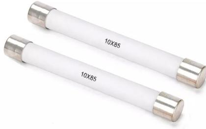
The 1500VDC Solar PV Fuse Link is specifically designed to protect PVsystems. This 10x85mm full-size cylindrical fuse securely protects 1500VDCPhotovoltaic (PV) systems. The 1500VDC 30A 10x85mm Solar PV Fuse Link is rated2A to 30A and meets the requirements of Photovoltaic (PV) applications such as PVstring, PV array protection, combiner box applications, etc.
