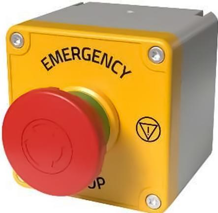
The ASI080TU0707-6GF12 is a compact, rugged emergency stop enclosure designed for industrial safety applications. Featuring a yellow polyamide housing with a red Ø 40 mm mushroom push-button and twist-to-release action, it ensures quick, secure operation in critical situations. The enclosure integrates 1 NO + 2 NC contact blocks and meets CE, UL, and CSA approvals.
