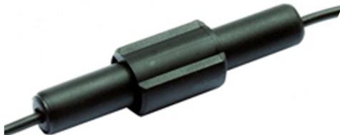
The PTF-80A is an inline fuse holder assembly that comes equipped with lead wires. The lead wires to this inline fuse holder are 18 AWG wire leads 150 mm long. This inline fuse holder is rated at 6.3 Amp at 250 Vac. The PTF-80A inline fuse holder features a locking design that once the fuse is inserted the unit stays together to ensure reliability. You can use either the 5x20mm or the 1 inch x 1/4 inch glass fuse in this inline fuse holder. Pack of 10.
