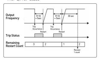
Speed search - When a fault occurs, the motor is normally rotating at a free-run state. In order to operate the system without any additional fault due to rotating motor, speed search feature needs to be activated.
