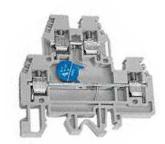
The **DAS.4V...** terminal blocks with varistor inserted as in **diagram 1**, limit voltage peaks due to surges, indirect atmospheric discharges and switching of inductive loads, and enable the equipment to pass the tests on immunity to electromagnetic interferences defined by the EN 61000-4-2 (Electrostatic discharge), EN 61000-4-4 (Fast Transient/Burst) and EN 61000-4-5 (Surge Test) Standards.
