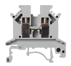
The ASI UK2.5N DIN Rail Terminal Block is a high-quality, compact solution for industrial wiring applications, providing secure wire connections with a screw clamp design. Engineered for control panels, automation systems, and power distribution, this terminal block is UL-listed and rated for 20A at 600V.
