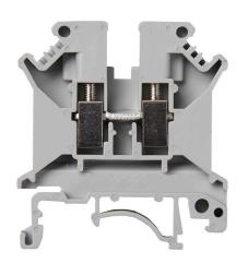
The ASI UK5N is a high-performance feed-through DIN rail terminal block engineered for reliability and efficiency in industrial and commercial wiring applications. UL-rated for 30A at 600V, this 6.2mm wide modular IEC terminal block accommodates a wire range of 30 to 10 AWG. Designed for universal compatibility, it mounts seamlessly on standard 35mm DIN rails and other rail types.
