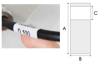
KM-ROLL wraparound cable markers are suitable for identifying wire or cable cables, tubes and conduit. The increased thickness of the label improves the handling and flexibility of the material, facilitating its application on the cable
