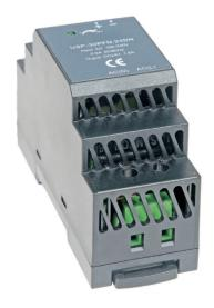
The USP-30PFN-24DN is a compact and efficient switching power supply, delivering a stable 24V DC output with an accuracy of ±2%. With a rated current of 1.5A and a maximum output power of 36W, this power supply is ideal for low-to-medium power applications. Its compact dimensions—just 35mm wide and 58mm high—make it perfect for space-constrained installations while ensuring consistent and reliable performance.
