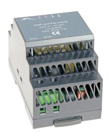
The USP-60PFN-24DN is a compact and efficient switching power supply designed for precision and reliability. With a DC output voltage of 24V and an accuracy of ±2%, this power supply delivers up to 60W of power with a rated output current of 2.5A. Its slim dimensions—just 52mm wide and 58mm high—make it an excellent solution for installations where space efficiency is essential, while ensuring dependable performance for a wide range of industrial and automation applications.
